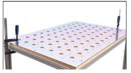
...and clamp it to your table frame. Two clamps are enough to secure it without hindering access from all sides.
