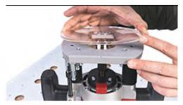
Attach the routing kit supplied with the product to your router to enable precise positioning of the holes.
